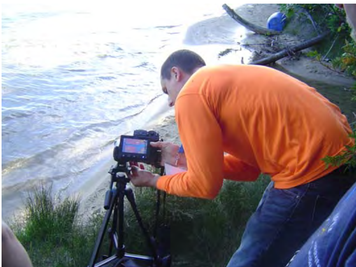
Martin Briggs demonstrating an infrared camera that shows the temperature difference between the warm lake water, and colder inflow from a stream and groundwater seeps. Photograph courtesy of Adam Heft.
