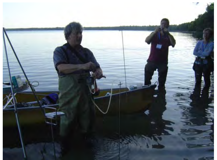
Mark Henry demonstrating pore water sampling devices near the shore of Higgins Lake. Photograph courtesy of Adam Heft.
