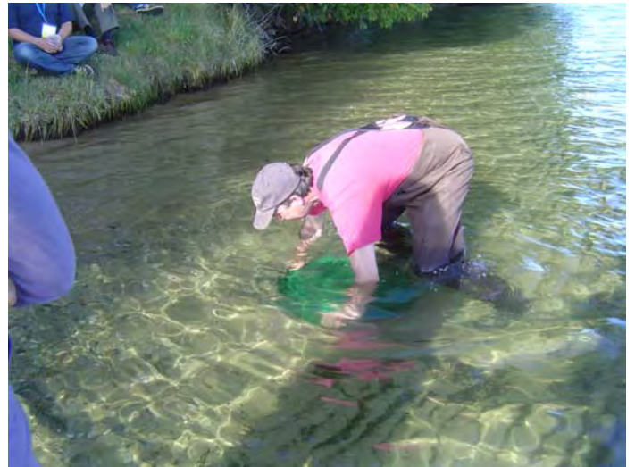
Brewster Conant demonstrating the installation of a seepage meter near the shoreline of Higgins Lake. Photograph courtesy of Rick Dunkin.
